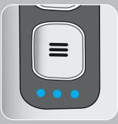
3. Indicator Lights will blink when charging. Unit is fully charged when all three lights stop blinking and remain fully lit. Remove the charging cable from unit.
